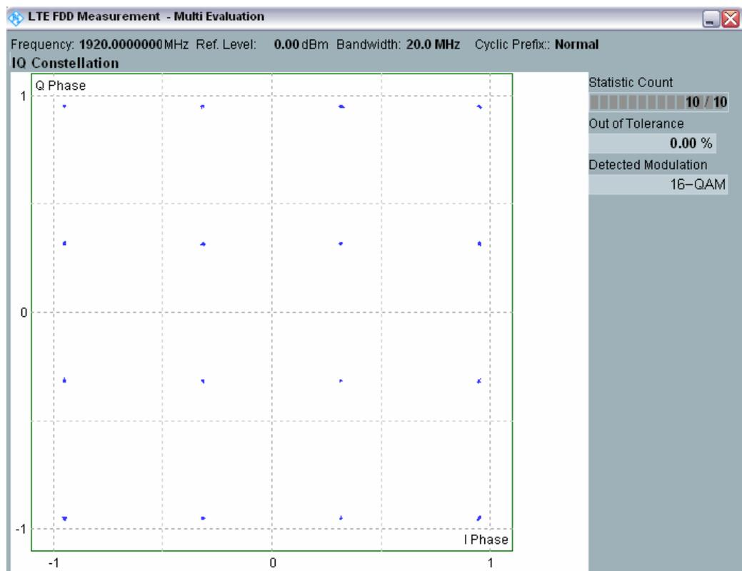
Fig. 3-6: LTE Multi Evaluation: I/Q Constellation diagram
