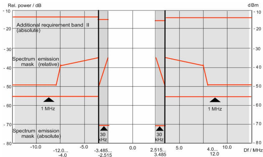
Fig. 3-4: Spectrum emission mask (WCDMA/FDD 3.84 MHz)
