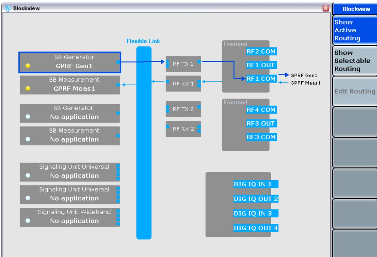
**Fig. 4-23: Blockview dialog - Active Routing**
