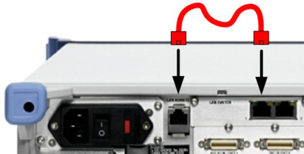
*Fig. 2-1: Ethernet connection between LAN SWITCH and LAN REMOTE connectors*
