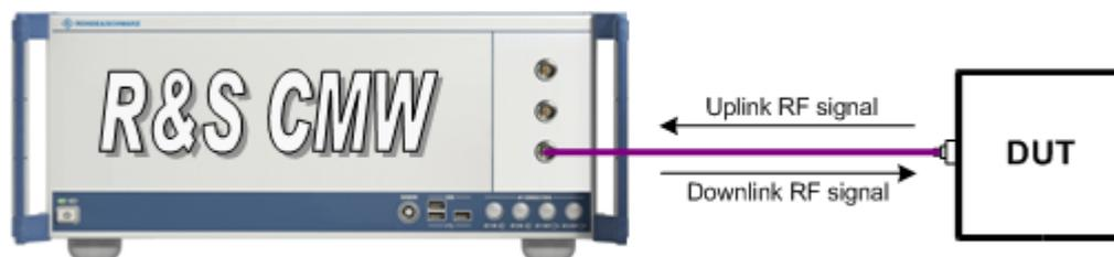
The RF connectors and other basic signal settings are configured in the "RF Settings" section at the beginning of the configuration dialogs. In contrast to generator or (TX) measurement applications, signaling applications provide output **and** input signal settings.
