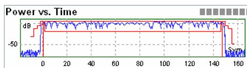
Fig. 3-3: Example of limit lines (GSM)
