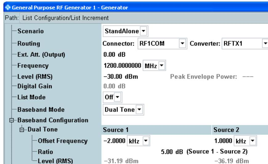
Fig. 2-2: General Purpose RF Generator dialog
