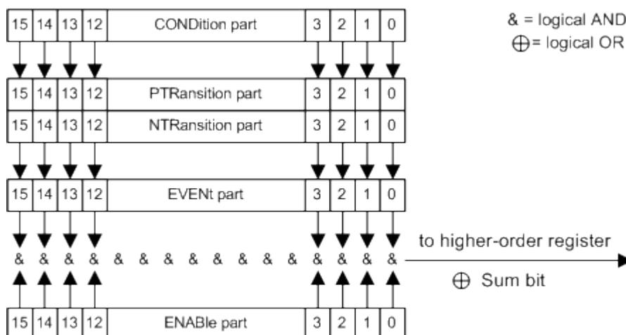
The sum bit is obtained from the EVENT and ENABLE part for each register. The result is then entered into a bit of the CONDITION part of the higher-order register.
